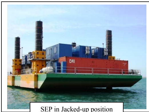
SEP in Jacked-up position (Bautino Bay)
